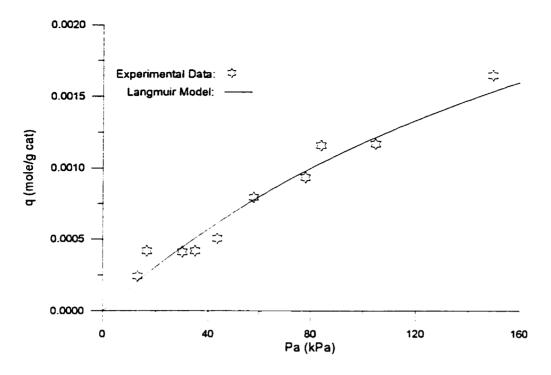
Figure E.3: Experimental observations and Langmuir Model at 160°C
