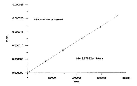
Fig C.2: Calibration of Isobutylene.
