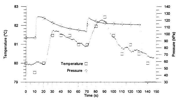
Fig 6.5: Temperature and Pressure Profile for Mode 3, Run 1. The first rise in pressure is the methanol injection and the second one the isobutylene injection.
