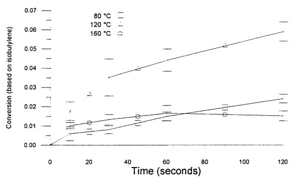
Figure 6.8: Conversion of Isobutylene toward MTBE for a Catalyst/Reactant ratio of 1. (The error bar correspond to the standard deviation)
