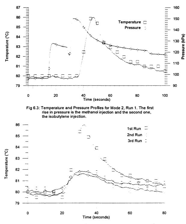
Fig 6.4: Comparison between the Temperature Profiles of the First three Runs after Regeneration for Mode 2
