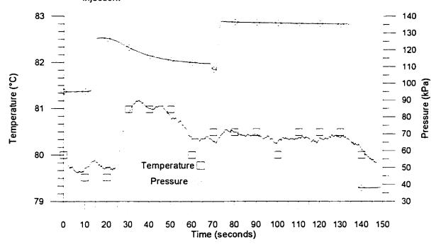
Fig 6.6: Temperature and Pressure Profiles for Mode 3, Run 3. The first rise in pressure is the methanol injection and the second one the isobutylene injection.
