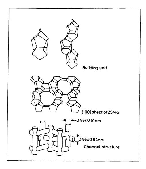
Fig 3.3: Structure of ZSM-5 Zeolite (from: Zeolite Catalysis: Principles and Applications, 1990).
