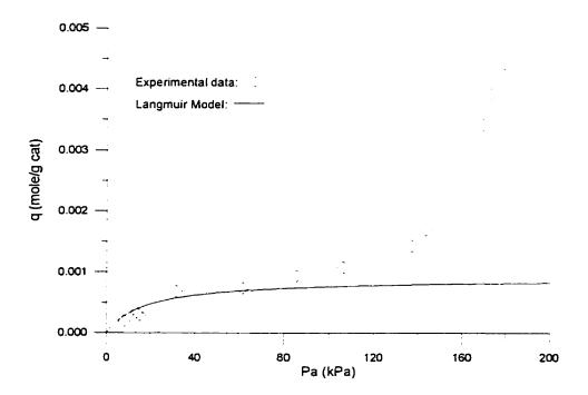
Figure E.2: Experimental observations and Langmuir Model at 120°C
