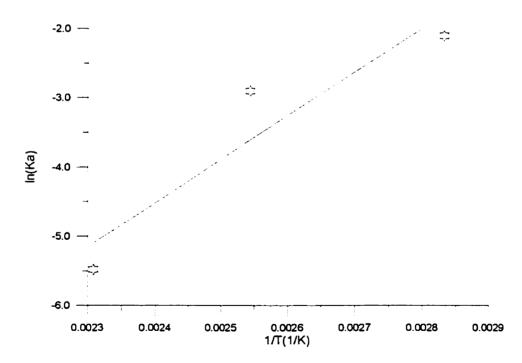
Figure E.4: Arhenius Plot of the adsorption constant (K<sub>A</sub>) against the inverse of temperature.
