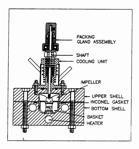
Figure 5.2: Schematic of the Riser Simulator
