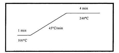
Fig 5.1 Temperature Program for the Poropak Q Column
