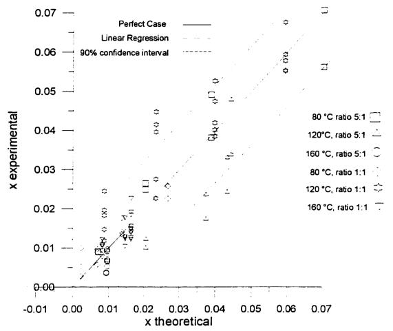
Fig 6.11: Comparison Between the Experimental and the Theoretical conversion.
