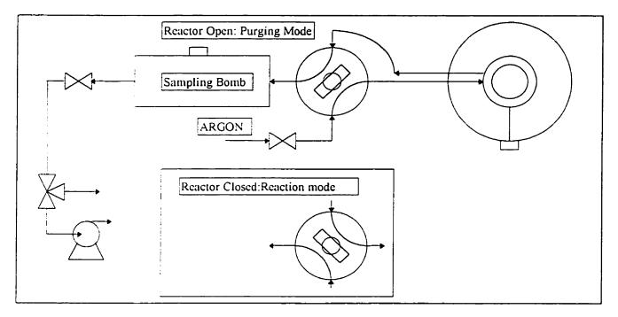
Figure 5.3: Schematic of the Sampling System
