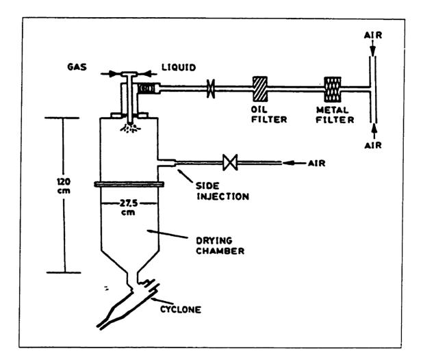
Fig 4.3: Schematic of the Spray Dryer available at CREC Laboratory.
