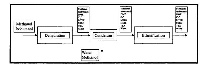
Figure 3.2: Schematic of the Two Reactor System: Dehydration Reactor and Etherification Reactor. (Nicolaides *et al.*, 1993)
