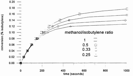
Figure 6.14 Effect of Changing the Methanol to Isobutylene Ratio on the Equilibrium Conversion and the Rate of Reaction (Wcat = 1 gram, Pmet = 28, Tr = 80 °C)
