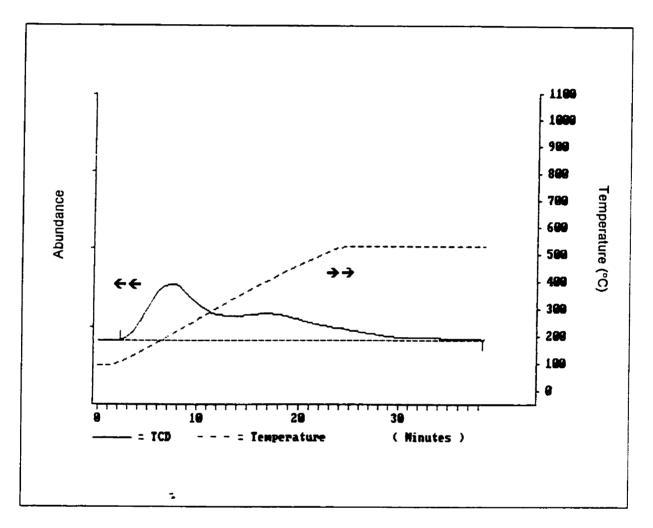
Fig 4.6 Results of the TPD Analysis of the H-ZSM-5
