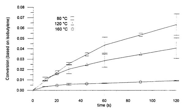
Figure 6.7: Conversion of Isobutylene toward MTBE for a Catalyst/Reactant Ratio of 5. (The error bars correspond to the standard deviation)
