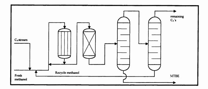
Figure 3.1: Typical Layout of a MTBE plant (Hutchings et al, 1992).
