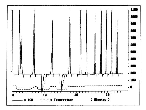
Figure A.3: Chromatogram of the BET Analysis of the Pelletized Zeolite.
