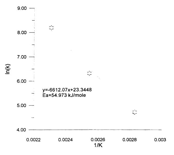
Fig 6.12: Arrhenius Plot of the Forward Kinetic Constant.
