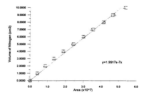
Fig A.5: Calibration of Nitrogen for the BET Analysis.
