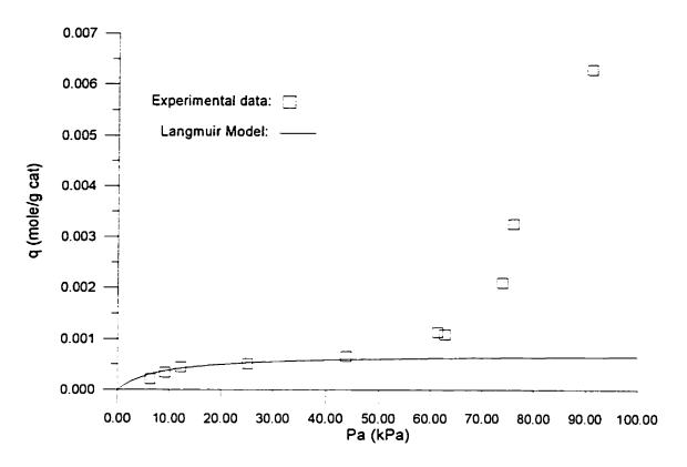
Figure E.1: Experimental observations and Langmuir Model at 80°C
