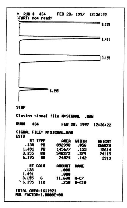
Figure C.5: Chromatogram of the example. The first peak is argon, the second methanol, the third isobutylene and the fourth MTBE
