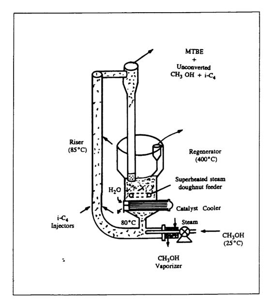
Figure 1.2: Schematic of the OXY-CREC Reactor Concept
