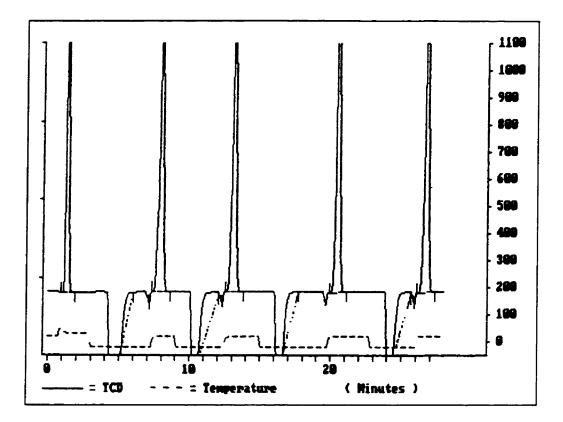
Figure A.1: Chromatogram of the BET Analysis of the Zeolite H-ZSM-5.
