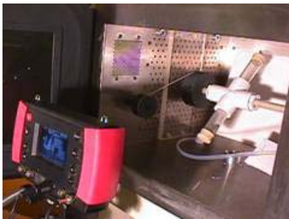
Figure 5.3 Motionmeter® enables frame by frame analysis of rapid events.
