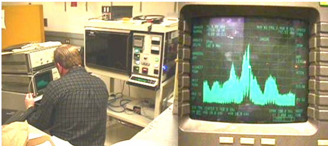
Figure 5.8 Signal peaking at 2.46 GHz (oven frequency) just above 60 dBm (~1kW).
