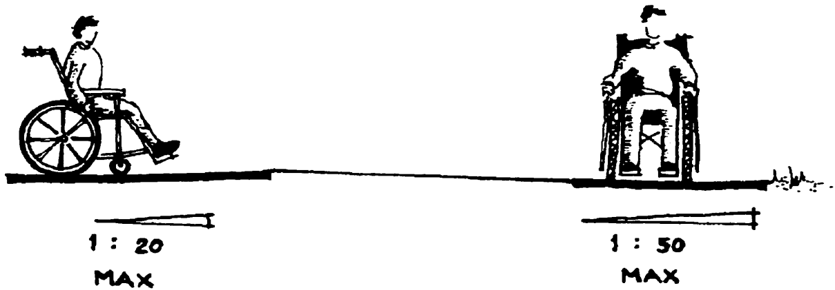
D. Recommended running slopes and cross slopes for pathways. (Canadian Heritage: Parks Canada, 1994: 17)
