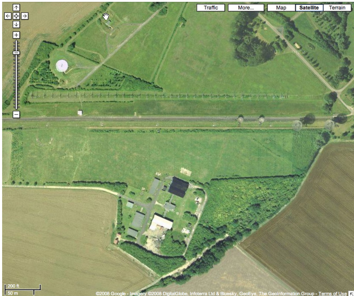
Figure 1.2 Satellite view of the Mullard Radio Astronomy Observatory (MRAO) near Cambridge, UK. The Interplanetary Scintillation Array, used for the pulsar discovery lies in the lawn field at the center between the buildings and the horizontal track, which is the 'One-Mile Telescope' used for aperture synthesis interferometry. Credit: Google Map.
