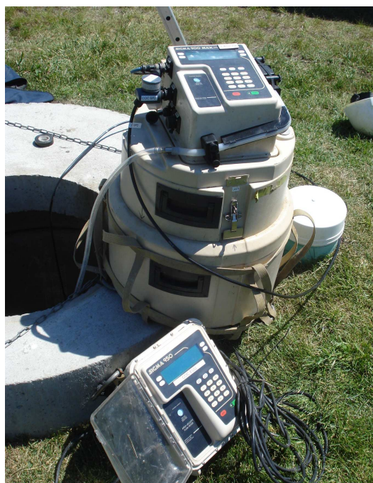
Figure 14: A Sigma 900 MAX auto-sampler and Sigma 950 flow-meter
