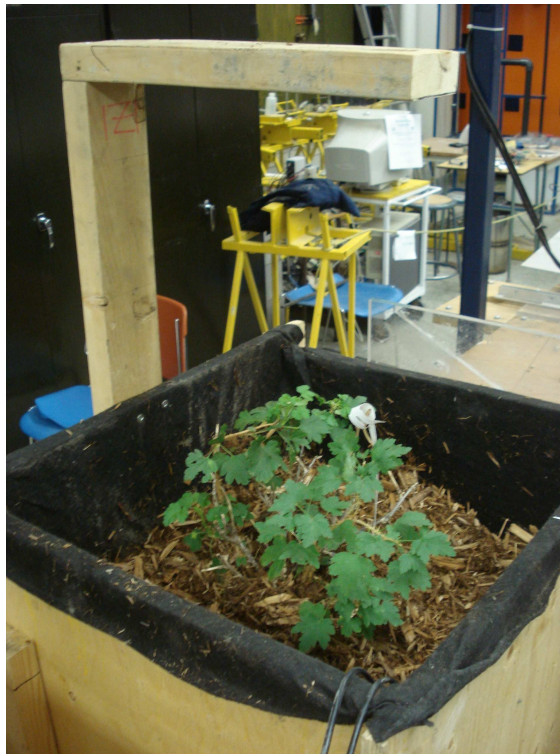
Figure 10: Complete column with shrub and mulch installed with a bracket for the stormwater runoff distribution system
