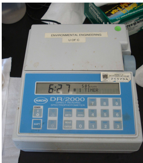
Figure 15: A HACH DR2000 Spectrometer, which was used for measuring water quality parameters
