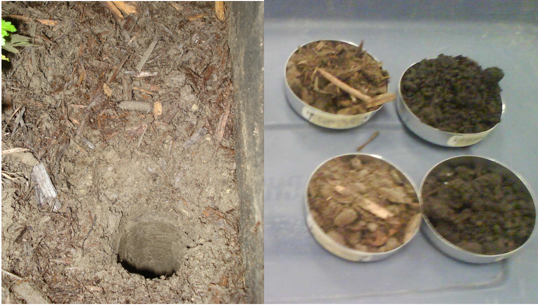
Figure 23: Bore hole for hydraulic conductivity measurement (L) and growing media samples (R)
