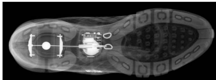
Fig. 5.2. X-ray image of the adidas\_1 in z-axis direction. Motor unit, regulating cable and the magnet are clearly visible.
