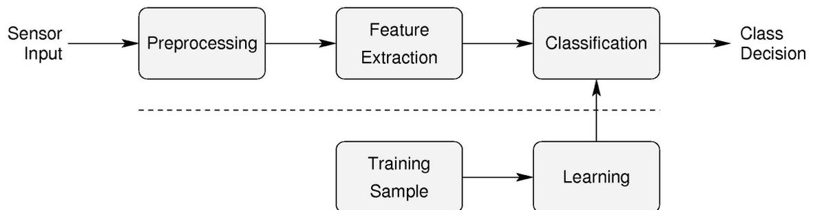
Fig. 1.1. Flow chart of a pattern recognition system (Niemann, 2003).
