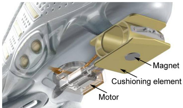
Fig. 6.1. The “adidas\_1” shoe, its cushioning element, magnet and motor unit (DiBenedetto et al., 2004; Eskofier et al., 2009a).
