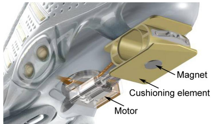
Fig. 5.1. A view of the adidas\_1 shoe, depicting the cushioning element and motor unit. The indicated magnet induces a magnetic field for compression measurement.
