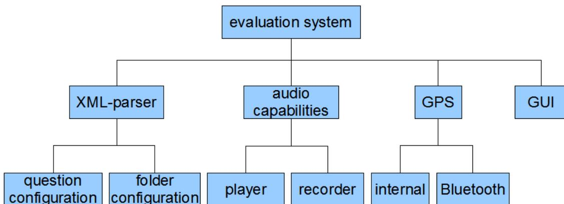
Fig. 7.3. Structural diagram of the software for the evaluation system.
