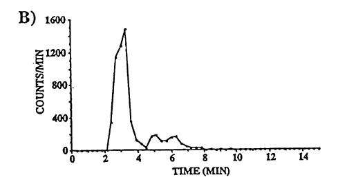
FIG. 2.4. Reverse-phase HPLC analysis of the reaction between 2-chloroacetyl chloride (0.5 mM) and GSH (5.0 mM) after 30 min. incubation at 25°C.
