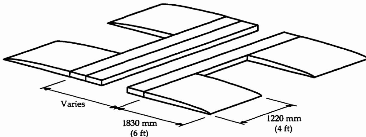
The full-scale field testing was carried out along Morningside Lane at the Central Experimental Farm in Ottawa. Morningside Lane has an asphalt surface and mountable concrete curb, and is 5.2 metres wide with about three percent crossfall. Due to the narrow width the test humps were centred over the crown of the road. The leading and trailing edges of the ramp sections were fastened to the pavement with concrete nails.
