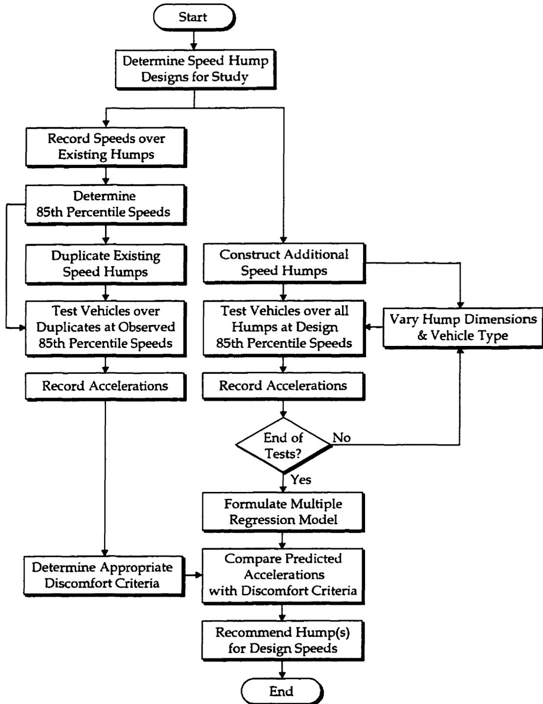
In the first phase of the experiment, speeds were recorded as motorists travelled over the existing 75 and 100 mm Watts and Seminole Profile speed humps. The 85th percentile hump-crossing speed for automobiles, and the mean speed for transit buses, were determined for each of the hump designs.
