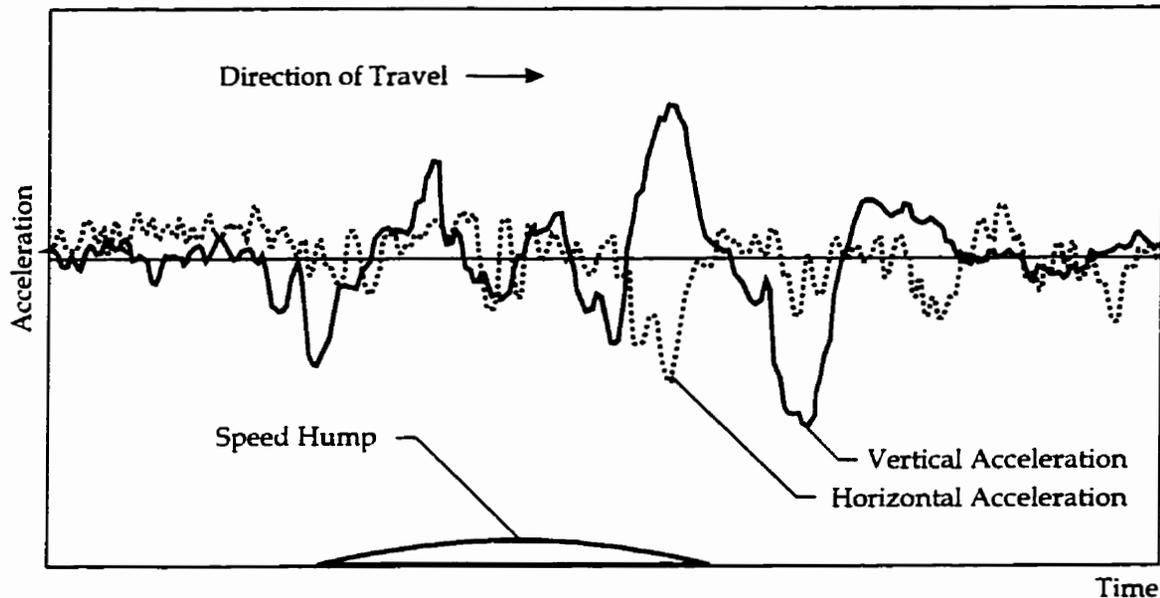
High amounts of vehicle noise and displacement were observed at 45 km/h with the Suzuki traversing the 4.9 m by 100 mm hump, and the transit bus traversing the 100 mm high Seminole Profile hump. There was no vehicle damage in either case, and the hump crossings appeared safe.
