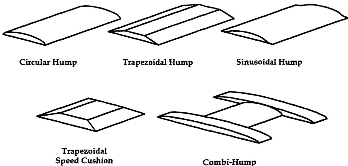
Speed *cushions* are raised sections of roadway limited in width to about 1.6 m, and were introduced in Germany in 1983 [Keller, 1986]. Automobiles must cross with at least one set of wheels on the cushions, but buses and wider vehicles can usually straddle them with only the inner wheels being affected. Cyclists can bypass the cushions, and bus speeds can be higher than with speed humps. As with humps, speed cushions vary in length, height and profile.
