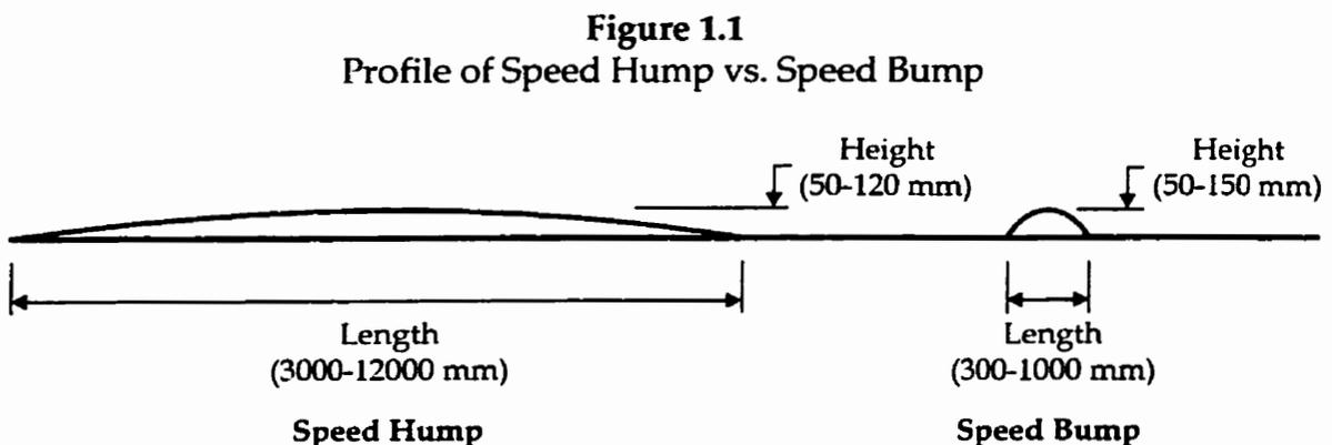
Speed humps are traffic calming measures. Traffic calming measures are physical design techniques that encourage or force motorists to drive at slow and constant speeds. They prevent speeding and can increase overall road safety. Traffic calming can also make streets more accessible and liveable for other users such as pedestrians, cyclists and nearby residents.
