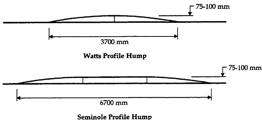
Both the Watts and Seminole Profile speed humps are proven designs. They can be easily constructed in the field, and present few maintenance problems.<sup>3</sup> The question was whether these specific humps are the best for Canadian conditions, or whether some variations on their design, featuring different lengths or heights, would prove more effective.
