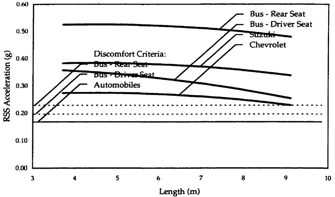
The optimal speed hump designs are summarized in Tables 7.5 and 7.6. The model predicted that humps designed to reduce transit bus speeds to 25 km/h will permit automobiles to traverse them at 35 km/h. The regression model was sensitive to small changes in discomfort levels, which could result in fairly wide ranges in lengths.
