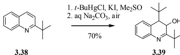
**Scheme 3.35.** Radical alkylation of 2-*tert*-butylquinoline to di-*tert*-butyl hydroquinoline **3.39** with the desired substitution pattern of **3.7** at the 2, 3 and 4 positions.
