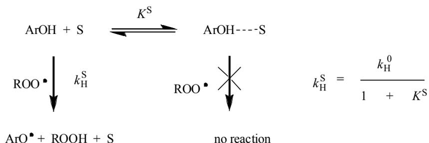
**Scheme 1.12.** Kinetic solvent effect on the reaction of phenols with peroxy radicals.<sup>60</sup>
