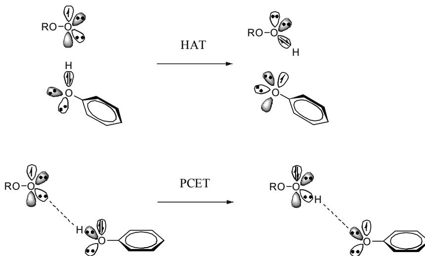
**Figure 1.1.** Hydrogen atom transfer mechanism versus proton coupled electron transfer mechanism.
