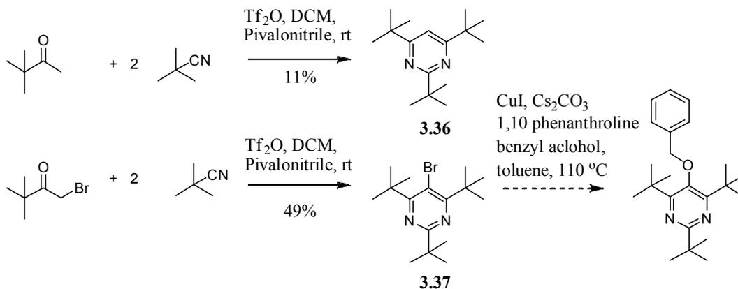
**Scheme 3.34.** *t*-Butylated pyrimidine synthesis using pyvalonitrile, (substituted) pinacolone and triflic anhydride.
