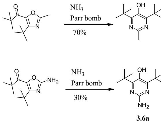
**Scheme 3.16.** Examples of oxazole ring opening reaction with ammonia and subsequent ring closing into target pyrimidinol **3.6a**.
