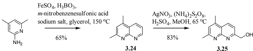
**Scheme 3.29.** Skraup reaction on 2-amino-4,6-dimethylpyridine resulting in 2,4-dimethyl-1,8-naphthyridine and its hydroxymethylation confirming radical alkylation methodology.
