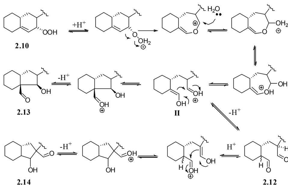
**Scheme 2.12.** Proposed mechanism for Hock cleavage of cholesterol 7 $\alpha$ -OOH in CDCl<sub>3</sub> to afford aldehydes **2.13** and **2.14**. Substituents are omitted on both the A and B ring of cholesterol for clarity, except the C ring residue at the 8 position.
