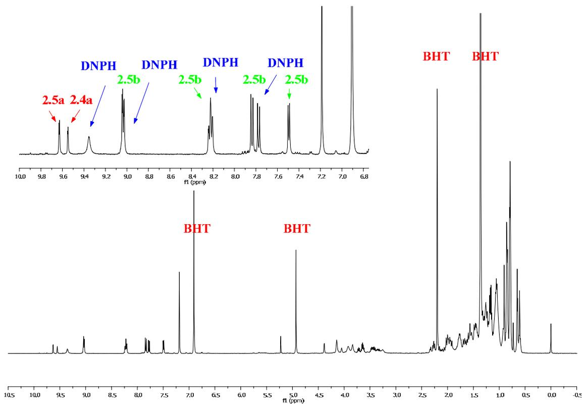
**Figure 2.11.**  $^1\text{H-NMR}$  spectrum of the mixture of **2.4a**, **2.5a**, **2.9** and **2.5b** in  $\text{CDCl}_3$  one minute after subjecting **2.7** to the DNPH derivatization conditions followed by work-up. Obtained at 500 MHz with chemical shifts reported in ppm relative to TMS.
