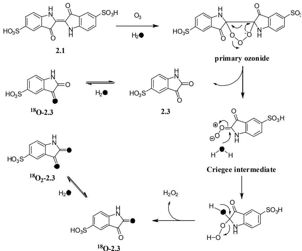
**Scheme 2.2.** Proposed mechanism of cleavage of indigo carmine (**2.1**) to two molecules of isatin sulfonic acid (**2.3**) with ozone in  $\text{H}_2^{18}\text{O}$ .
