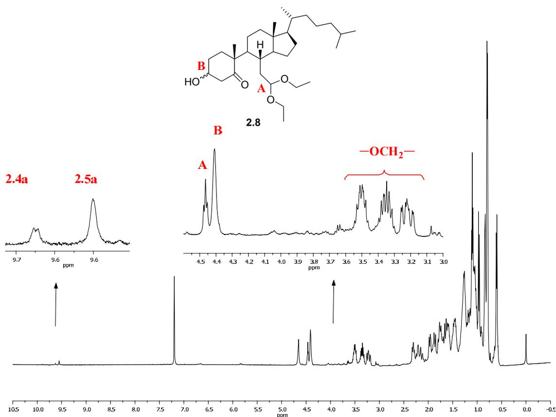
**Figure 2.5.** <sup>1</sup>H-NMR spectrum of **2.8**, the acetal derived from **2.4a**, in CDCl<sub>3</sub>. Note that some **2.5a** is formed due to aldolization of **2.4a** upon acetalization. Obtained at 500 MHz with chemical shifts reported in ppm relative to TMS.
