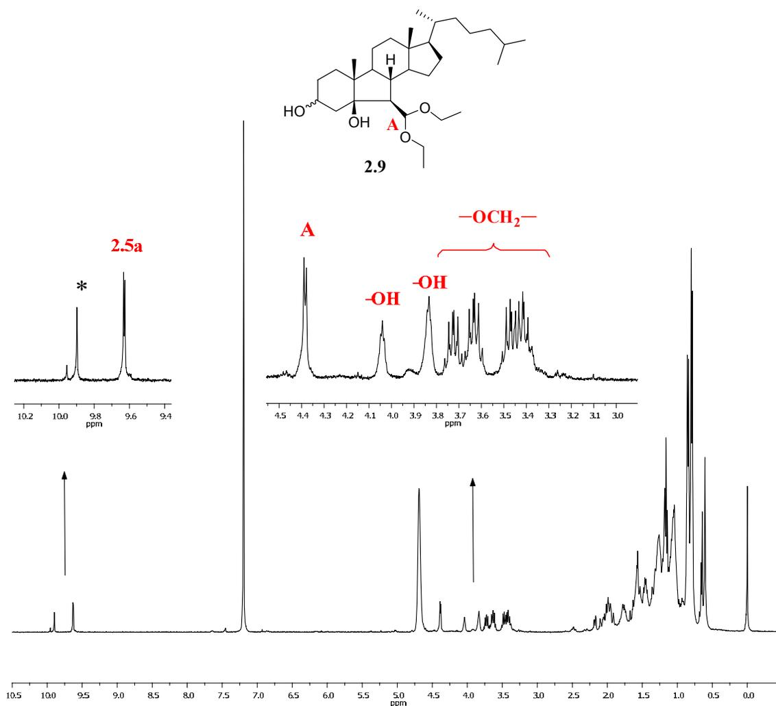
**Figure 2.6.**  $^1\text{H-NMR}$  spectrum of **2.9**, the acetal derived from **2.5a** in  $\text{CDCl}_3$ . Note that some dehydration product (\*) is formed on treatment of **2.5a** with acid for acetalization (confirmed by LC/MS *vide infra*). Spectrum obtained at 500 MHz with chemical shifts reported in ppm relative to TMS.
