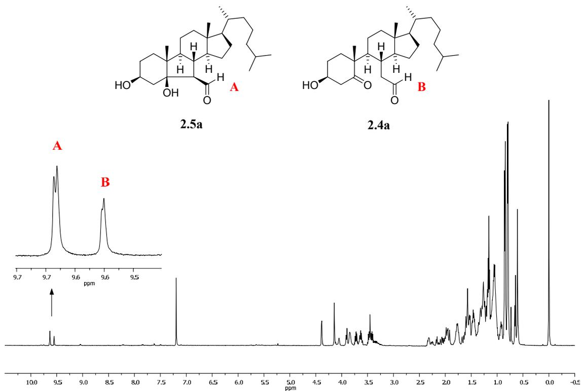
**Figure 2.4.**  $^1\text{H-NMR}$  spectrum of the reaction products obtained from treatment of **2.7** with HCl (conc.) in EtOH, analyzed after workup. Obtained at 500 MHz in  $\text{CDCl}_3$  with chemical shifts reported in ppm relative to TMS.
