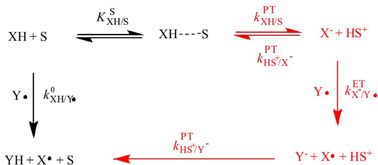
**Scheme 1.13.** SPLET mechanism in red versus HAT mechanism in black.
