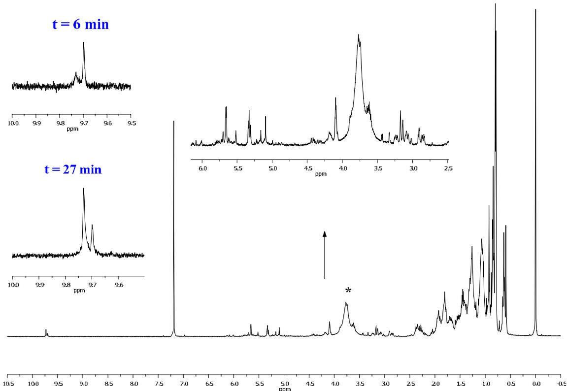
**Figure 2.17.**  $^1\text{H}$ -NMR spectrum of chol  $7\alpha$ -OOH in  $\text{CDCl}_3$  following treatment with TFA (2.7 mM). Insets show aldehydes peaks distribution at  $t = 6$  minutes and  $t = 27$  minutes. Obtained at 500 MHz with chemical shifts reported in ppm relative to TMS. (\* =  $\text{H}_2\text{O}$ ).
