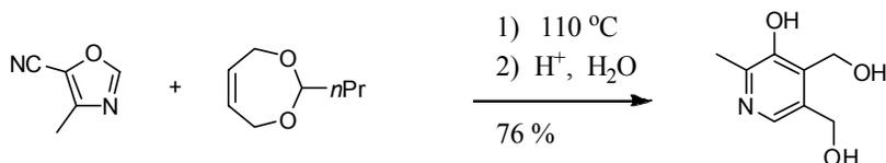
**Scheme 3.3.** Synthesis of vitamin B<sub>6</sub> from 4-methyloxazole-5-carbonitrile and (Z)-4,7-dihydro-2-propyl-1,3-dioxepine through a hetero Diels-Alder reaction.
