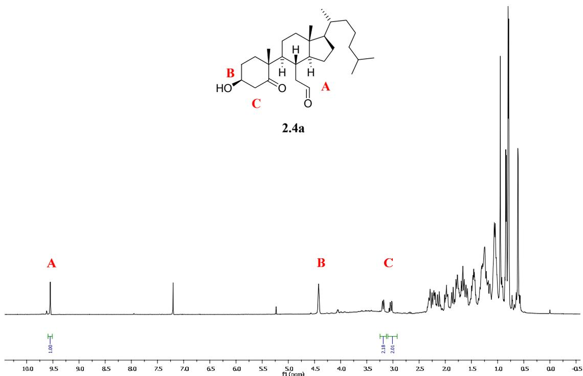
**Figure 2.3.**  $^1\text{H}$ -NMR spectrum of the cholesterol 5,6-secosterol **2.4a** in  $\text{CDCl}_3$ . Obtained at 500 MHz with chemical shifts reported in ppm relative to TMS. Note that some **2.5a** is formed due to aldolization of **2.4a** in the NMR sample.
