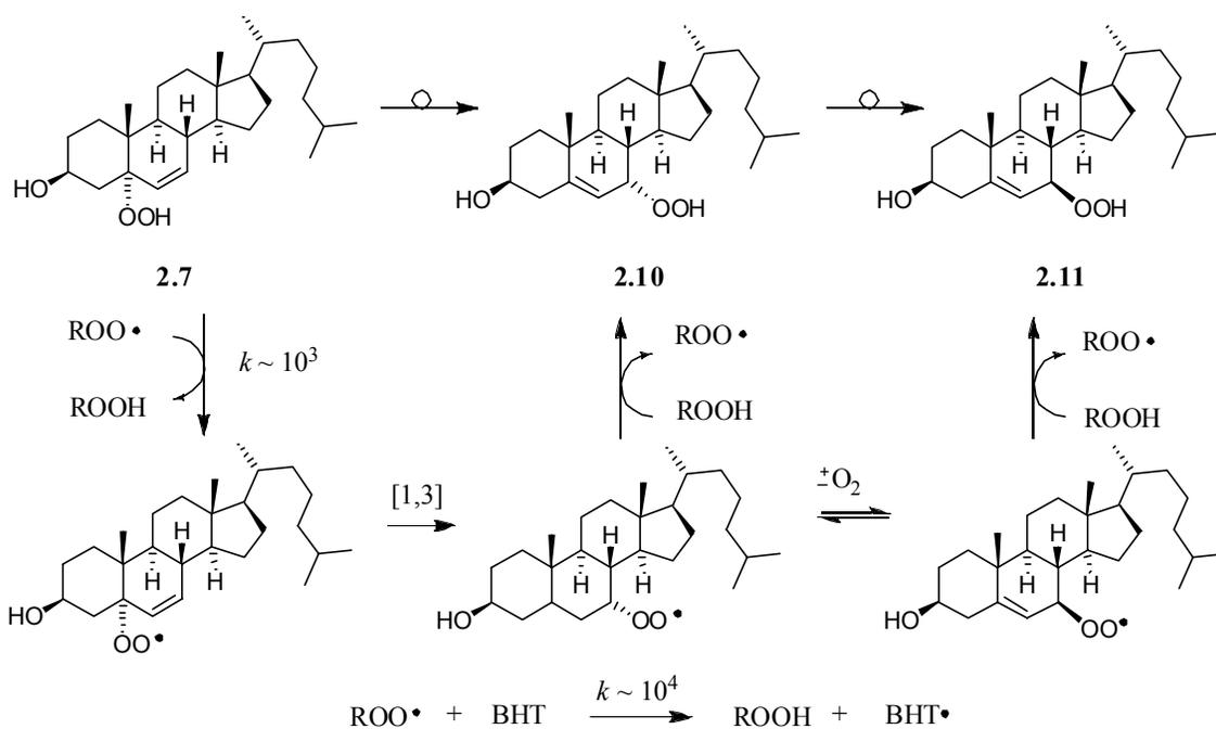
**Scheme 2.11.** Rearrangement of cholesterol 5 $\alpha$ -OOH **2.7** in non-hydrogen bonding solvent to cholesterol 7 $\alpha$ -OOH **2.10** which can epimerize to cholesterol 7 $\beta$ -OOH **2.11**. Both processes involve allylperoxy radicals and as such are inhibited by antioxidants such as 2,6-di-tert-butyl-4-methylphenol, BHT.
