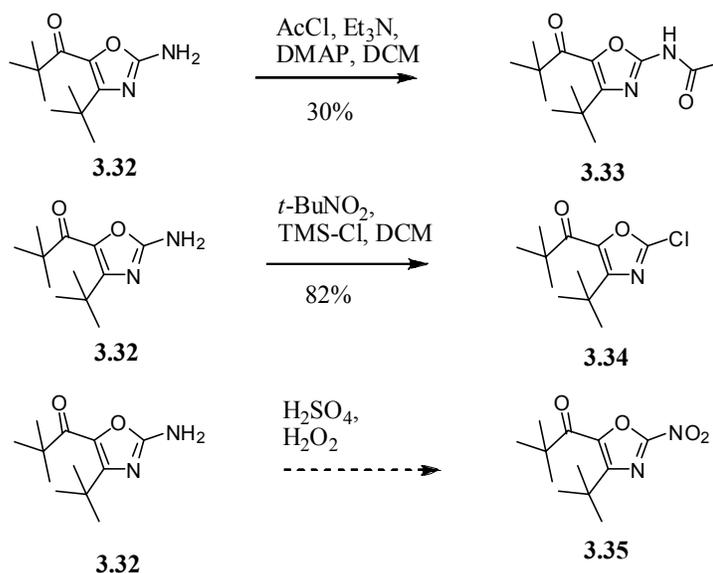
**Scheme 3.33.** Acetylation, chloro-diazotization and oxidation of oxazole **3.32**.
