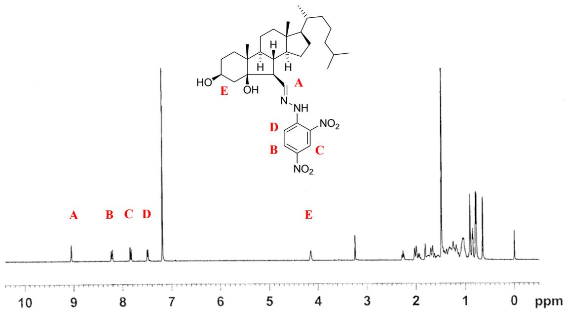
**Figure 2.15.** <sup>1</sup>H-NMR spectrum of authentic DNPH derivatized secosterol **2.5b**. Obtained at 500 MHz with chemical shifts reported in ppm relative to TMS.
