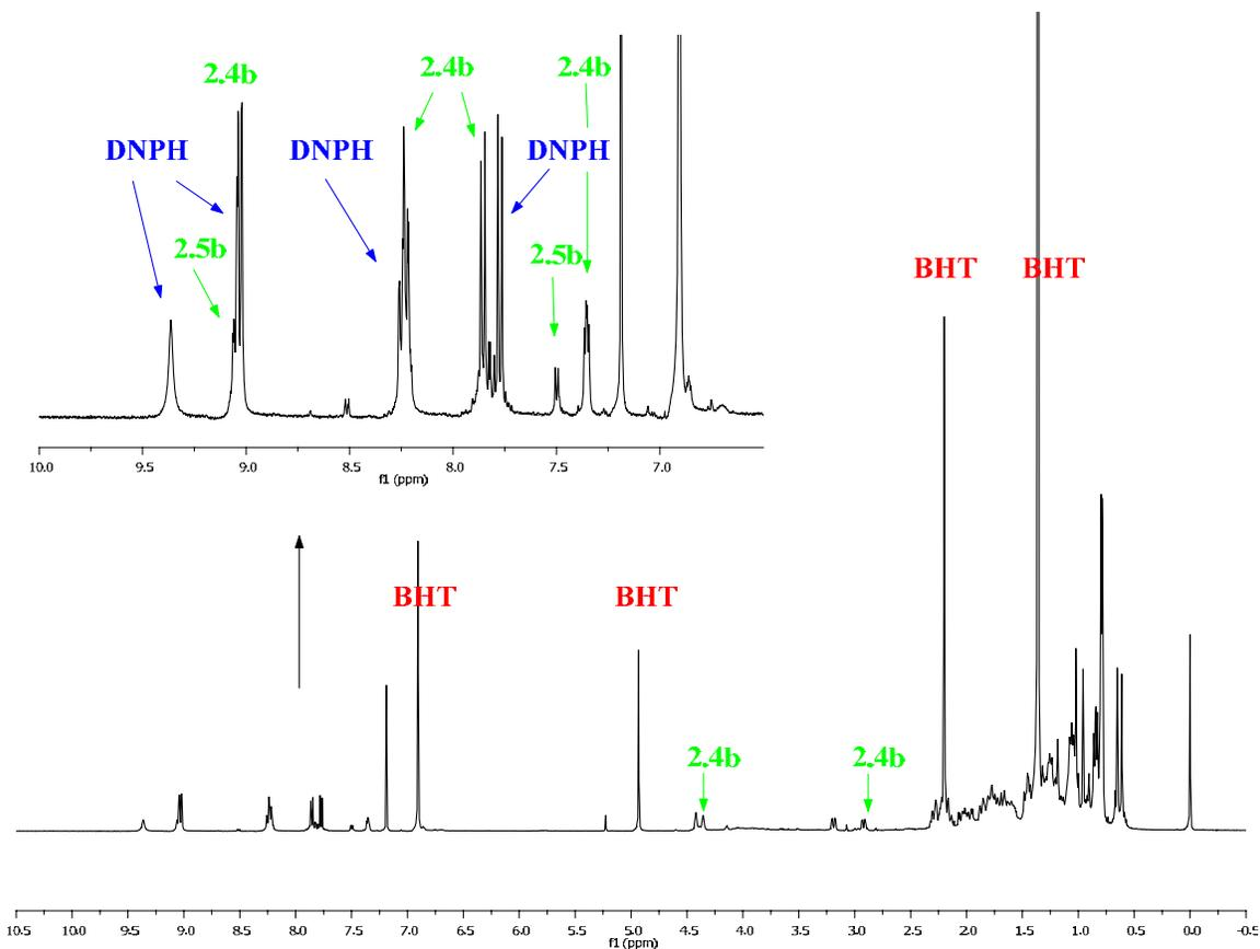
**Figure 2.13.** <sup>1</sup>H-NMR spectrum of the mixture of **2.4b** and **2.5b** in CDCl<sub>3</sub> 2 hours after subjecting **2.4a** to the DNP derivatization conditions followed by work-up. Obtained at 500 MHz with chemical shifts reported in ppm relative to TMS.
