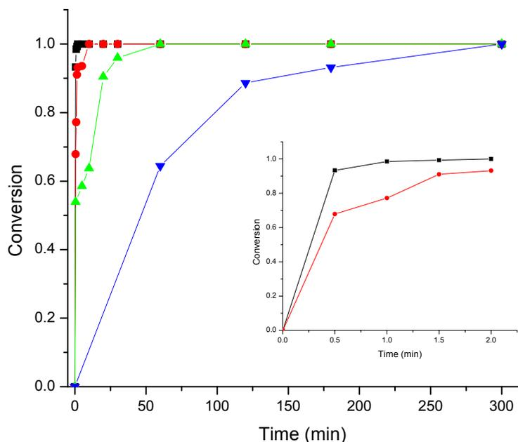
**Figure 2.8.** Conversion of cholesterol  $5\alpha$ -OOH (4,8 mmol/ml in EtOH) to **2.4a** and **2.5a** as a function of time at different concentrations of HCl (■, 0.1 M; ●, 0.01 M; ▲, 0.001 M; ▼, 0.0001 M).
