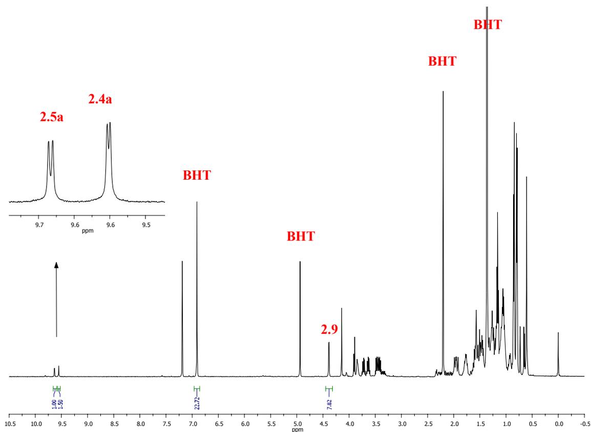
**Figure 2.7.**  $^1\text{H-NMR}$  spectrum of the mixture of **2.4a**, **2.5a** and **2.9a** formed upon treatment of **2.7** with HCl in EtOH. Obtained at 500 MHz with chemical shifts reported in ppm relative to TMS.
