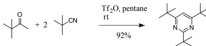
**Scheme 3.17.** Termolecular synthetic approach to access tri-*tert*-butylated pyrimidine ring system.
