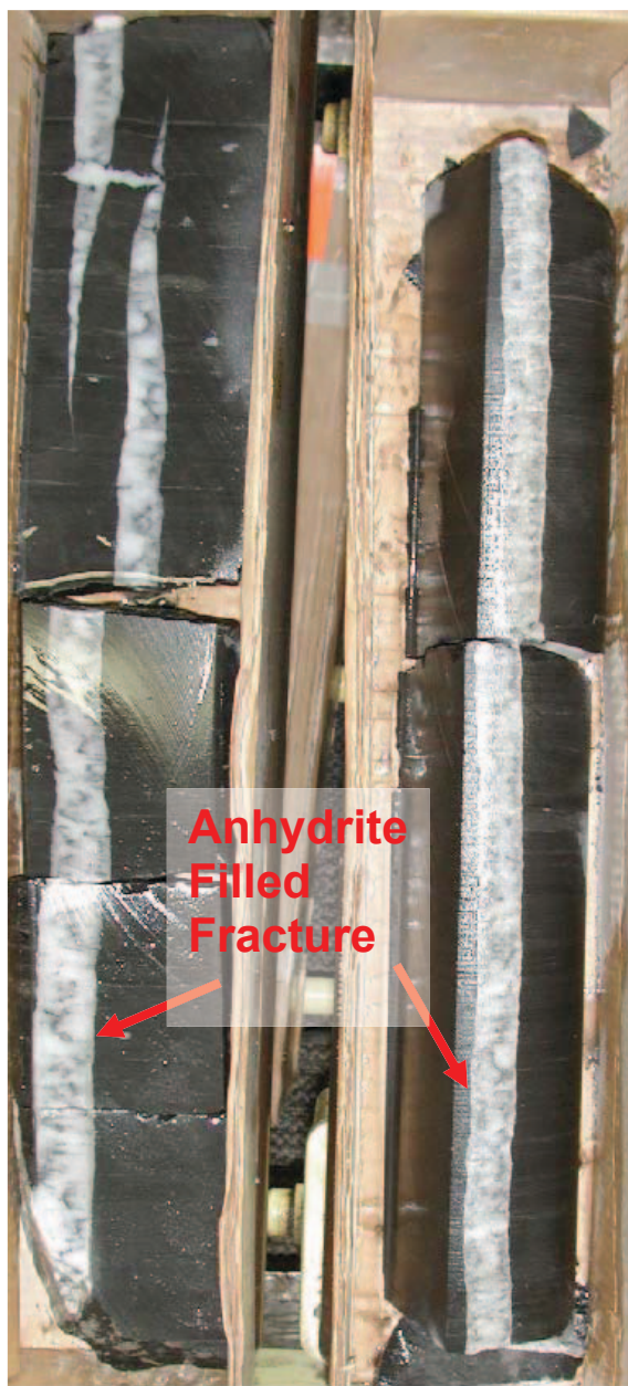
Figure 3.12 – Sharp walled fracture seen within black horizontally laminated shale of the Doig Formation. Fracture displays minor sub cm offsets (fault?) and is interpreted to have occurred after some lithification of surrounding shale. This feature is an indication of active tectonism (or fault reactivation) within the study area. Core is approximately 3 inches wide. 10-36-70-10W6, 2568m.
