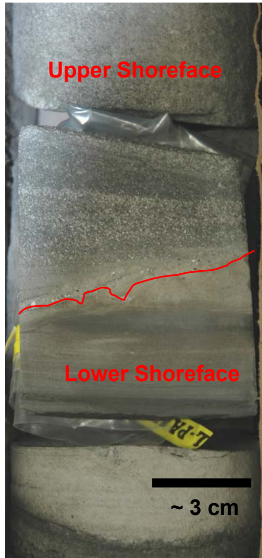
Figure 3.08 - Marine firmground surface in well 11-17-66-6W6 at 2783.0m depth. Sharp erosional scour separates fine grained laminated lower shoreface sediments from overlying cross bedded upper shoreface sediments. Facies change across erosional scour suggests that approximately five metres of sediment has been removed if thickness comparisons of shoreface interval are made with adjunct wells.
