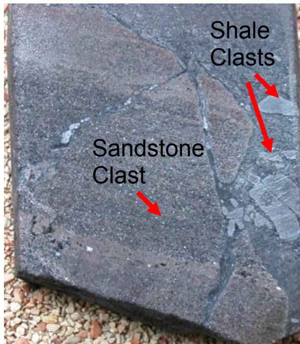
Figure 2.05 - Fractured lithified sandstone clast at the base of tidal channel. Note fractures within sandstone clast indicating semi-lithification at time of transport (lower-left) and shale rip-up clasts (middle-right). Core width is approximately 9 cm wide. (6-15-69-9W6, 2631m)
