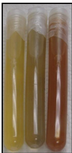
Figure S4.3. Digital photographs of: A) autoclaved cells and Tl-jarosite, B) Tl-jarosite and S. putrefaciens and C) cell-free Tl-jarosite at 893 hours
