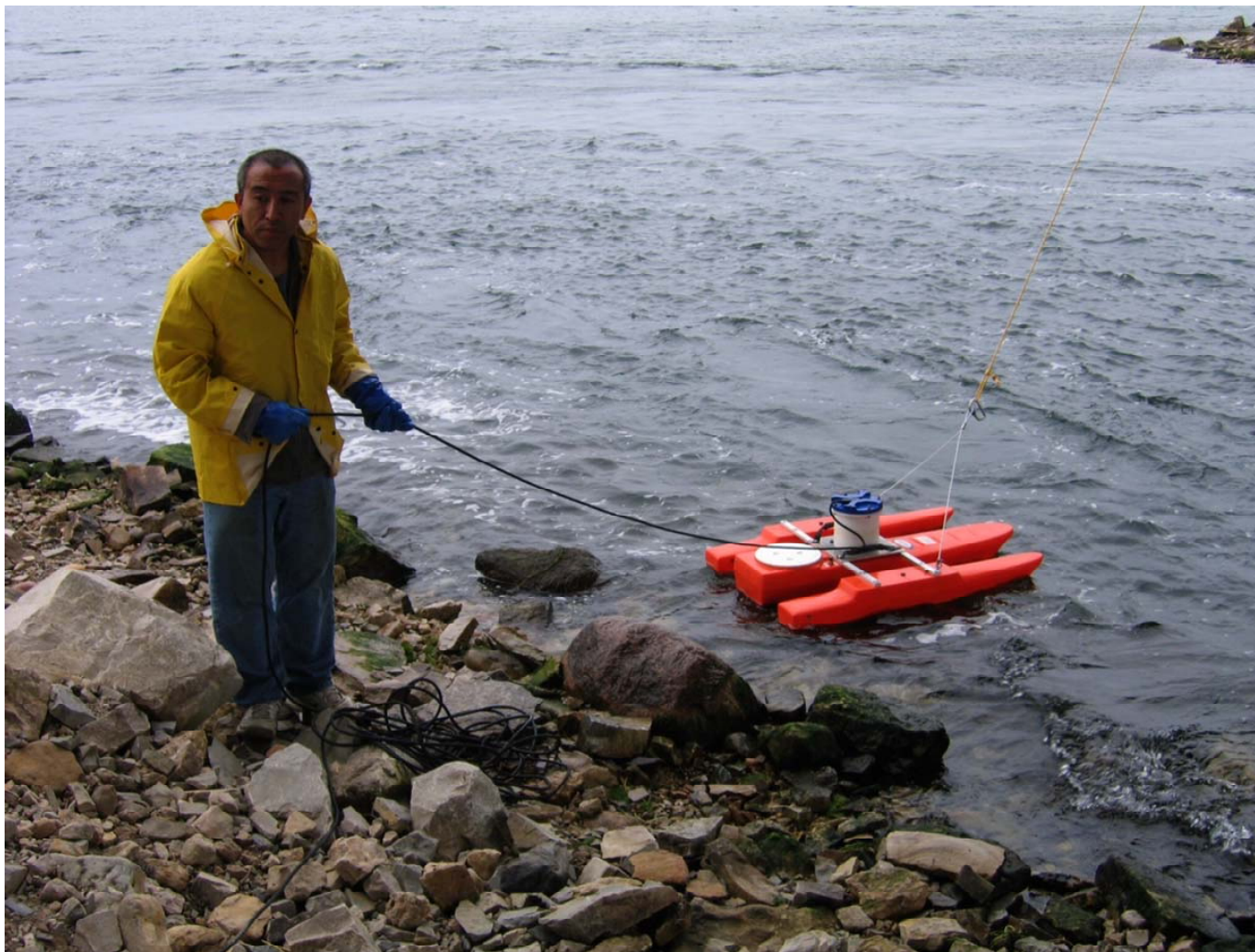
Figure 4 Acoustic Doppler Current Profiler mounted in a catamaran
