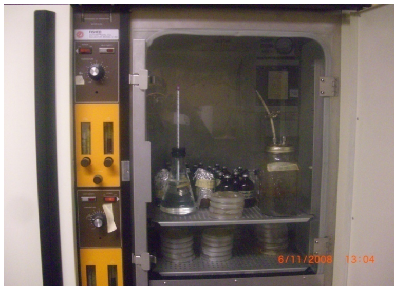
Figure 4. 1: Maintenance of T. versicolor on Agar Plates in an Incubator, Fisher Isotemp® Dual CO 2 incubator Model 413D.
