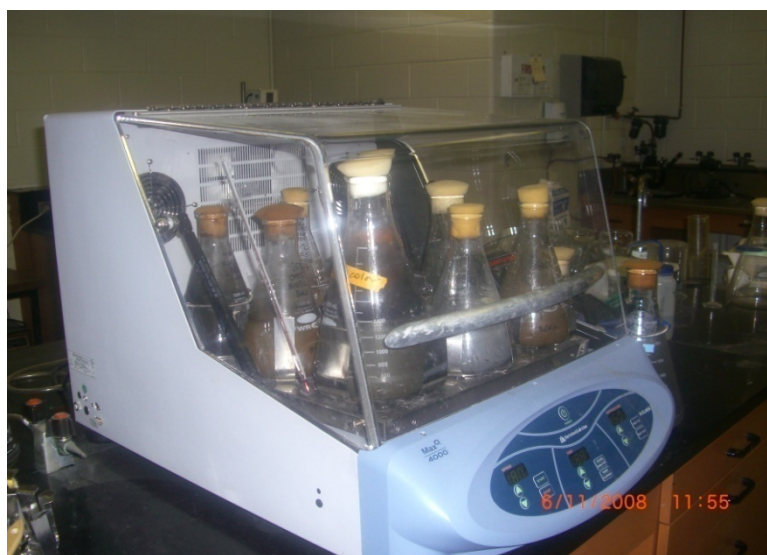
Figure 4.2: Microbial Cultures in Contact with Samples in Erlenmeyer Flasks mounted on an Orbital Shaker, Barnstead Max Q .
