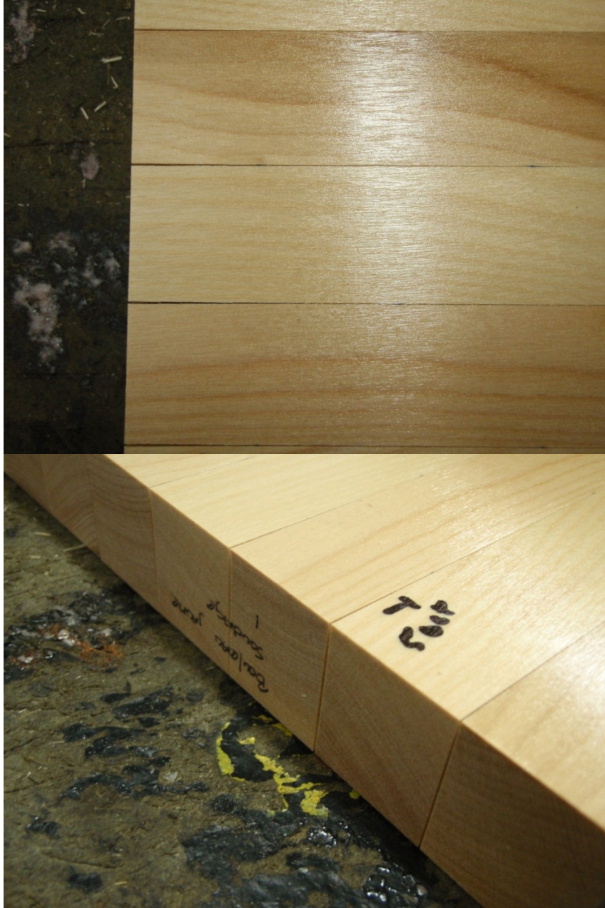
Figure 4.11 Edge separation along the length of a wood-welded panel after 24h at 20 °C and 20% RH.
