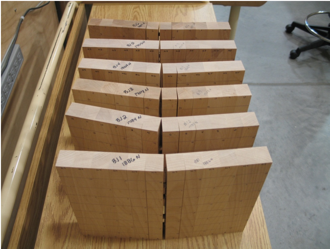
Figure 4.8 Failure of a wood-welded panel in the joints at the midspan or in the lamination next to it following bending tests.
