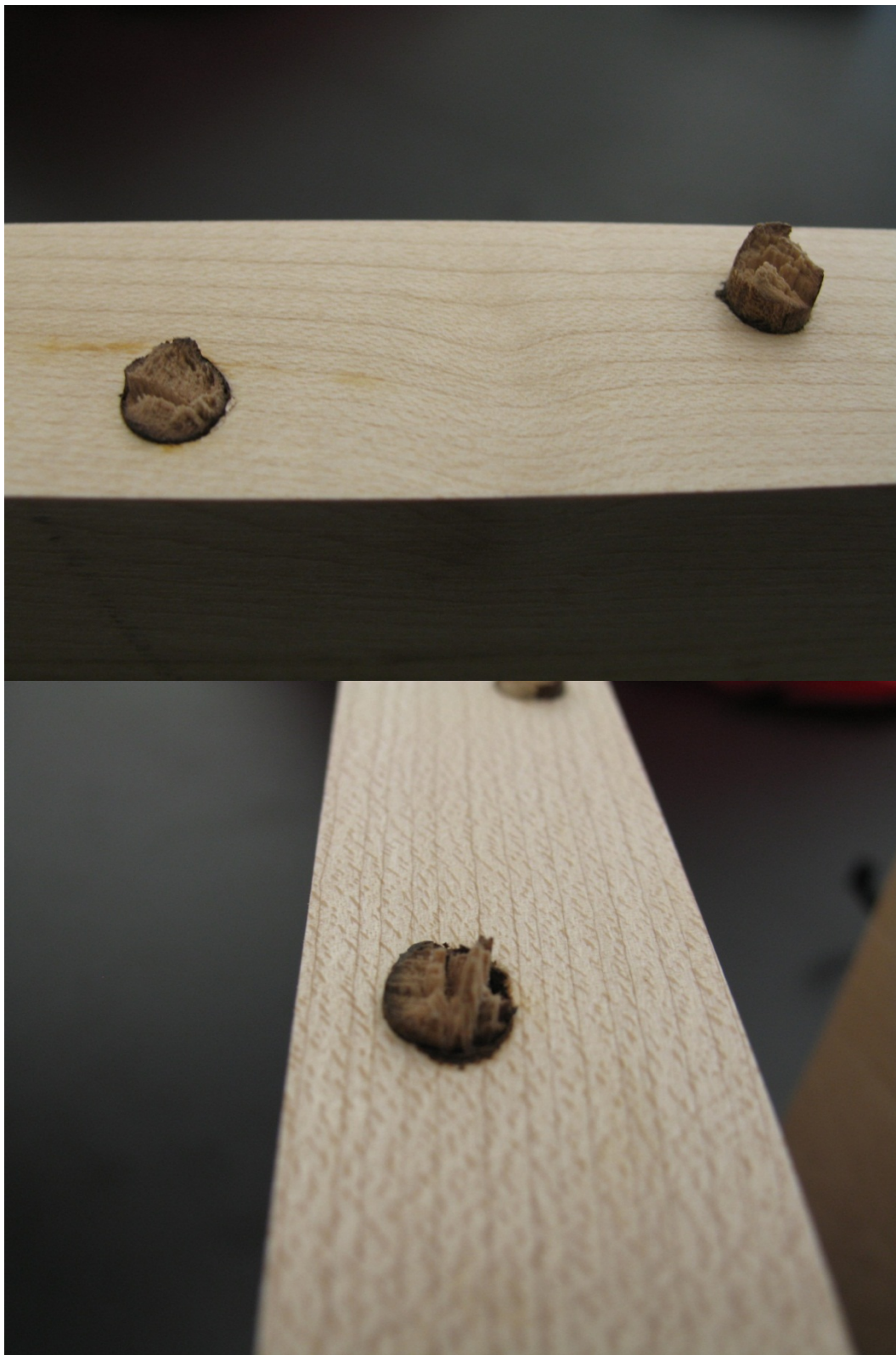
Figure 4.9 Fractured dowels with no slippage along the welded interface.
