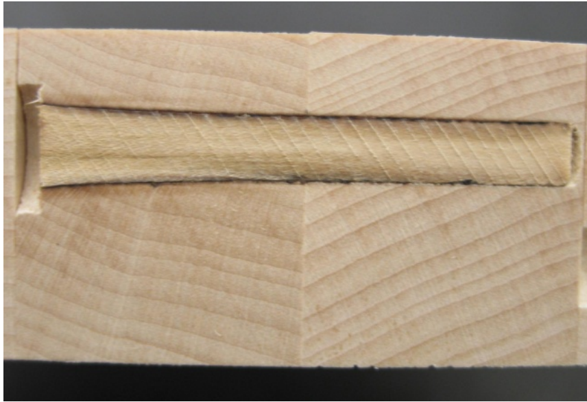
Figure 4.2 Cross-cut wood dowel welded through two wood slats.
